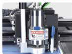
Water cooling frequency conversion main shaft
